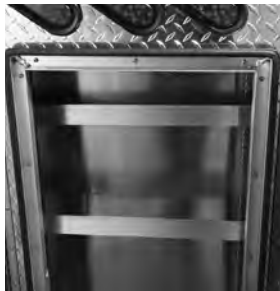
Chain hangers in each side compartment
