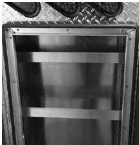
Chain hangers in each side compartment
